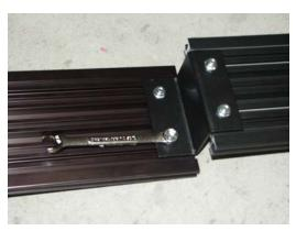
Attach the extrusion adapter bracket to the 12" section of extrusion using (2) 1/4" x 3/4" bolts and serrated nuts.
